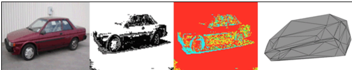
Figure 19: Original, intensity, and range image information, with extracted convex hull of a parked car (Teizer et al., 2005)
